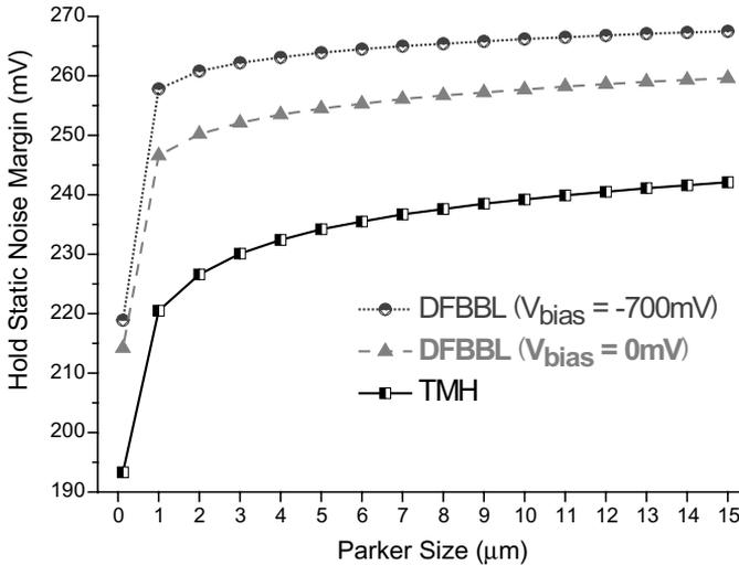
Fig. 14. The hold static noise margins of the TMH and DFBBL flip-flops with different Parker sizes.  $T = 90^\circ\text{C}$ . The minimum Parker size on the  $X$  axis is  $0.12 \mu\text{m}$ .
