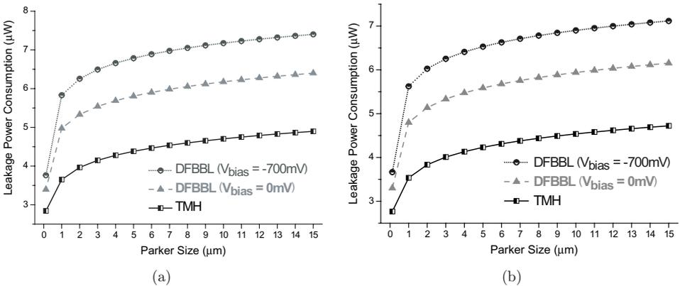
Fig. 9. The leakage power consumed by the TMH and DFBBL shift registers with different Parker sizes.  $T = 90^\circ\text{C}$ . (a) Stored data = “0”. (b) Stored data = “1”. The minimum Parker size on the X axis is  $0.12\ \mu\text{m}$ .
