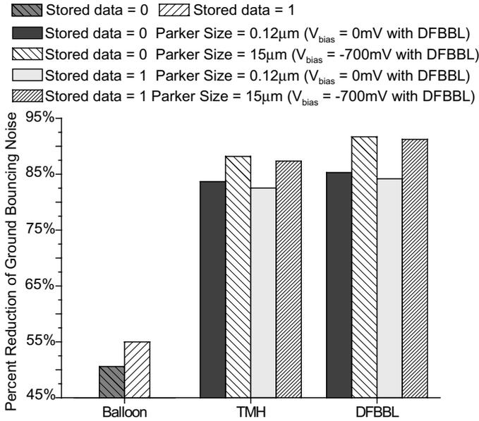
Fig. 8. Percent reduction of ground bouncing noise produced with different MTCMOS circuit techniques as compared to the conventional Mutoh technique at 90°C.
