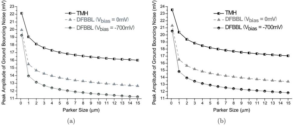
Fig. 6. The peak ground bouncing noise produced by the TMH and DFBBL shift registers with different Parker sizes.  $T = 90^{\circ}C$ . (a) Stored data = “0”. (b) Stored data = “1”. The minimum Parker size on the X axis is  $0.12 \mu m$ .
