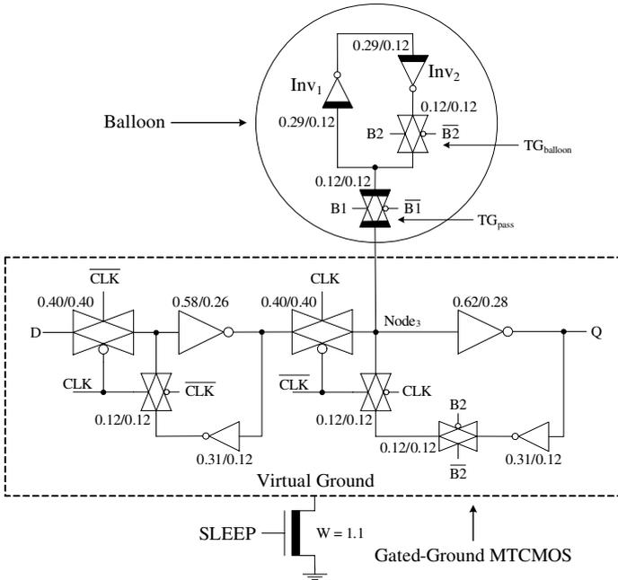
Fig. 3. Low-leakage Balloon MTCMOS flip-flop (Balloon-FF) with data preserving sleep mode.<sup>4</sup> High- $|V_{th}|$  transistors are represented with a thick line in the channel region. The transistor sizes ( $W_{PMOS}/W_{NMOS}$ ) are in micrometers assuming an 80 nm CMOS technology. All the channel lengths are minimum ( $L = 80$  nm).
