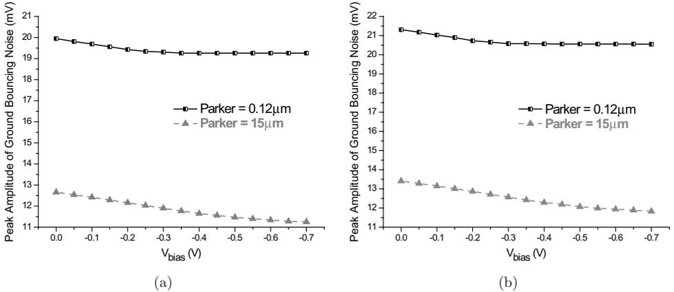
Fig. 7. The peak ground bouncing noise produced by the DFBBL shift register at different  $V_{bias}$ .  $T = 90^{\circ}C$ . (a) Stored data = “0”. (b) Stored data = “1”.
