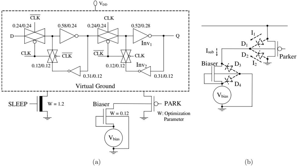
Fig. 5. Proposed sequential MTCMOS circuit with dynamic-forward-body-biased Parker (DFBB). (a) The tri-mode MTCMOS flip-flop with a dynamic-forward-body-biased low- $|V_{th}|$  Parker (DFBBL). (b) The proposed dynamic forward body bias generator for the Parker. High- $|V_{th}|$  transistors are represented with a thick line in the channel region. The transistor sizes ( $W_{PMOS}/W_{NMOS}$ ) are in micrometers assuming an 80 nm CMOS technology. All the channel lengths are minimum ( $L = 80$  nm).
