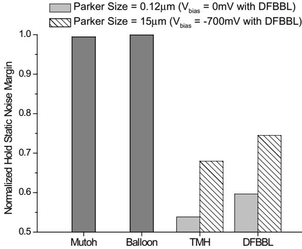
Fig. 16. The hold static noise margins of different MTCMOS circuit techniques normalized to the hold SNM of the Balloon-FF.  $T = 90^\circ\text{C}$ .
