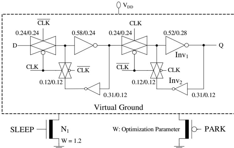
Fig. 4. Standard tri-mode MTCMOS flip-flop with zero-body-biased high- $|V_{th}|$  Parker (TMH).<sup>6</sup> High- $|V_{th}|$  transistors are represented with a thick line in the channel region. The transistor sizes ( $W_{PMOS}/W_{NMOS}$ ) are in micrometers assuming an 80 nm CMOS technology. All the channel lengths are minimum ( $L = 80$  nm).
