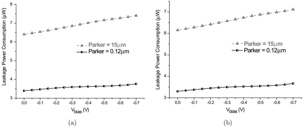
Fig. 10. The leakage power consumed by the DFBBL shift register at different  $V_{\text{bias}}$ .  $T = 90^{\circ}\text{C}$ . (a) Stored data = "0". (b) Stored data = "1".
