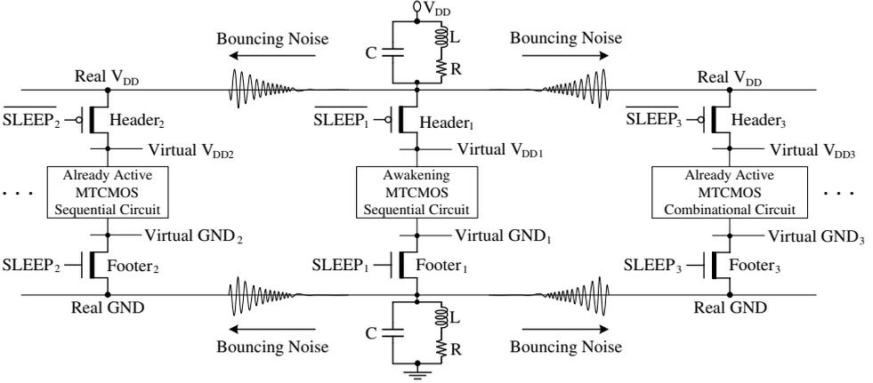
Fig. 1. A conventional multi-domain MTCMOS circuit with multiple autonomous low- $|V_{th}|$  circuit blocks with individual distributed sleep transistors. High- $|V_{th}|$  sleep transistors are represented with a thick line in the channel region.  $SLEEP_1 : 0 \rightarrow V_{DD}$ .  $SLEEP_2 = SLEEP_3 = V_{DD}$ .
