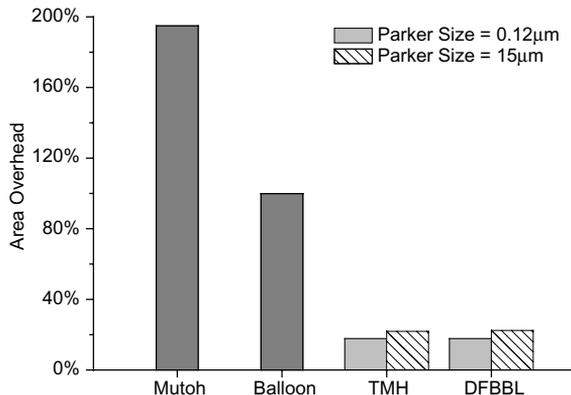
Fig. 13. The area overhead with different MTCMOS circuit techniques as compared to the standard single low- $|V_{th}|$  shift register.
