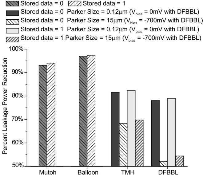
Fig. 11. Percent leakage power reduction provided by different MTCMOS circuit techniques in the sleep mode as compared to the standard single low- $|V_{th}|$  shift register.
