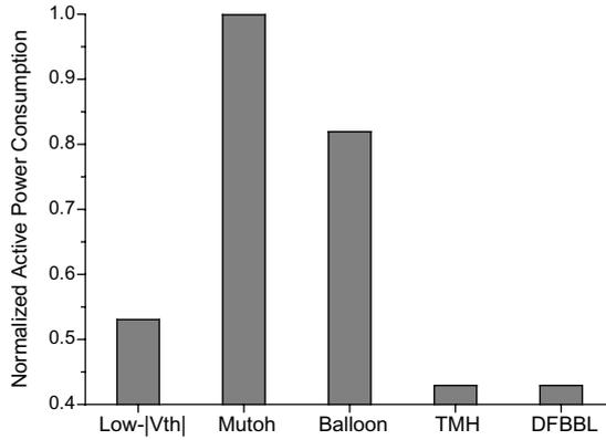
Fig. 12. The active power consumption with different circuit techniques normalized to the Mutoh shift register.  $T = 90^{\circ}\text{C}$ .
