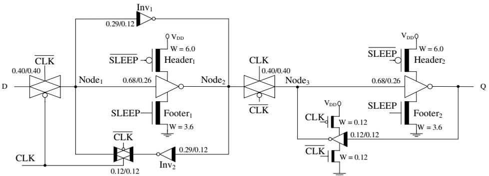
Fig. 2. The conventional MTCMOS flip-flop (Mutoh-FF) with data preserving sleep mode.<sup>2,3</sup> High- $|V_{th}|$  transistors are represented with a thick line in the channel region. The transistor sizes ( $W_{PMOS}/W_{NMOS}$ ) are in micrometers assuming an 80 nm CMOS technology. All the channel lengths are minimum ( $L = 80$  nm).
