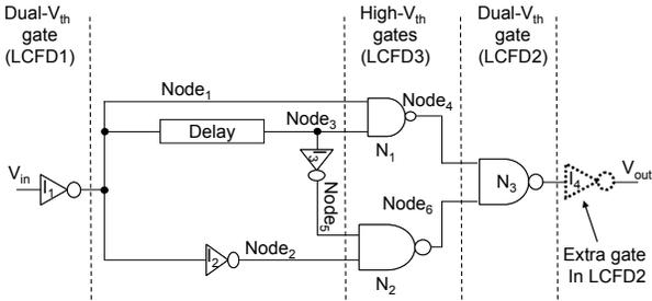
Fig. 7. Proposed hybrid level-converter/frequency-doubler. The dual- $V_{th}$  gate(s) and all the downstream gates after the dual- $V_{th}$  gate(s) operate with  $V_{DDH}$ .
