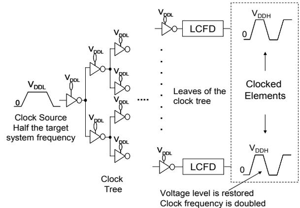
Fig. 6. The proposed dual- $V_{DD}$ /dual-frequency clock distribution technique. LCFD: hybrid level-converter/frequency-doubler.  $V_{DDL}$ : low optimum supply voltage that minimizes the clock skew.  $V_{DDH}$ : nominal higher supply voltage required by the clocked elements for high speed.
