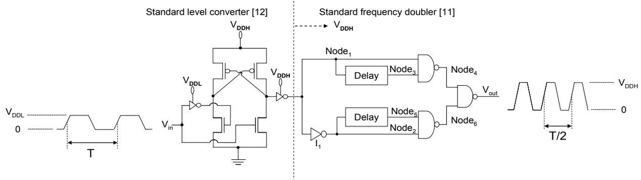
Fig. 11. A standard single- $V_{th}$  cascaded two-stage level-converter/frequency-doubler circuit.
