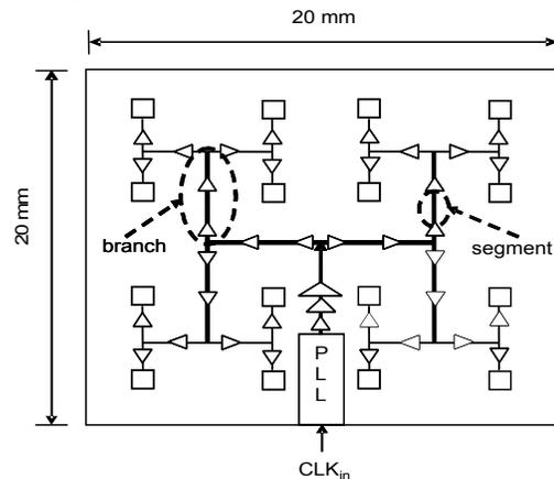
Fig. 1. Two level buffered H-tree clock distribution network.
