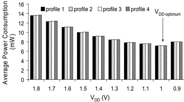
Fig. 5. Average power consumption of the clock distribution network versus the supply voltage for four different temperature profiles.
