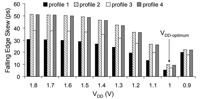
Fig. 4. Temperature fluctuations induced clock skew (for the falling edge) versus the supply voltage.  $V_{DD-nominal} = 1.8V$ .
