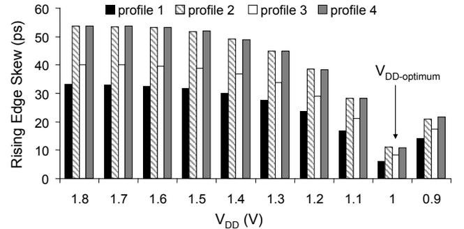
Fig. 3. Temperature fluctuations induced clock skew (for the rising edge) versus the supply voltage.  $V_{DD-nominal} = 1.8V$ .
