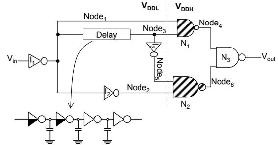
Fig. 10. LCFD3. The shaded NAND gates have high- $V_{th}$  transistors. The shaded inverters have high- $V_{th}$  NMOS transistors.
