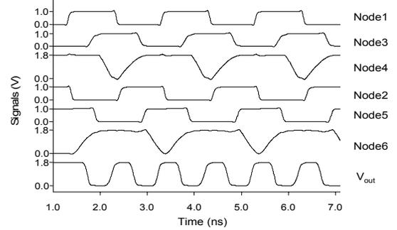
Fig. 8. Voltage waveforms of the frequency doubler ( $T = 25^\circ C$ ).
