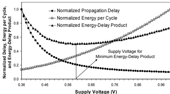
Fig. 6. Normalized energy, delay, and energy-delay product as a function of the supply voltage at the room temperature (25°C) for a 16-bit Brent-Kung adder.
