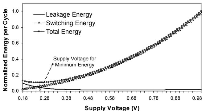
Fig. 4. Normalized total, switching, and leakage energy as a function of the supply voltage at 25°C for a 16-bit Brent-Kung adder.
