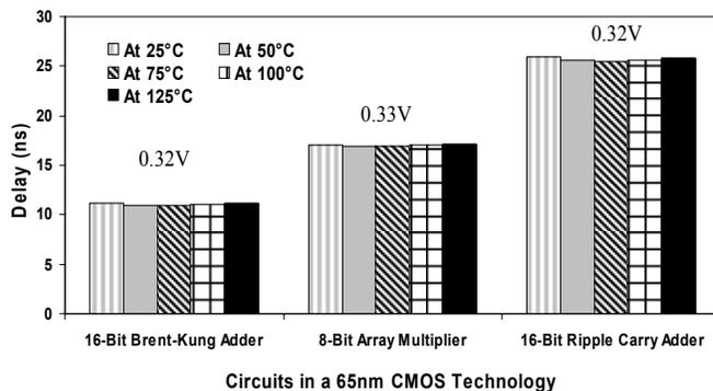
Fig. 3. Optimum supply voltages that achieve temperature variation insensitive speed characteristics.
