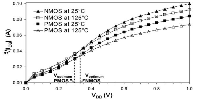
Fig. 1. Variation of MOSFET drain current ( $I_{DS}$ ) with supply voltage ( $V_{DD}$ ) and temperature in a 65nm CMOS technology.  $|V_{DS}| = |V_{GS}| = V_{DD}$ .
