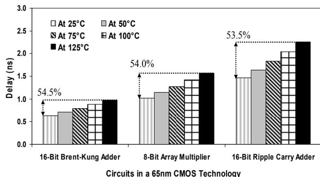
Fig. 2. Percent delay variation with temperature for circuits operating at the nominal supply voltage ( $V_{DD} = 1.0V$ ).
