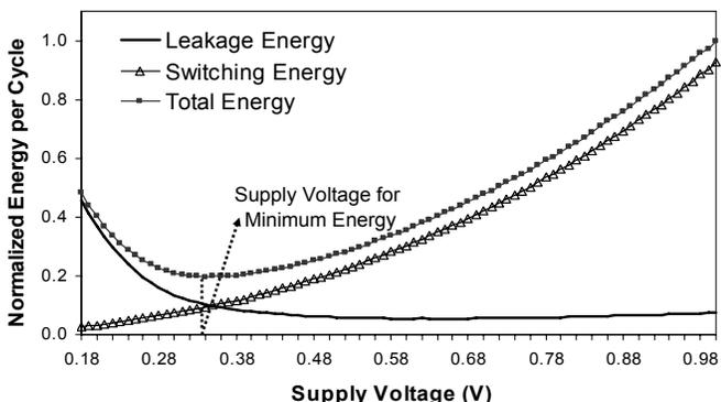
Fig. 5. Normalized total, switching, and leakage energy as a function of the supply voltage at 125°C for a 16-bit Brent-Kung adder.
