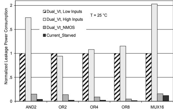
**Fig. 8. Comparison of total leakage power consumed by domino circuits with the three circuit techniques at 25 °C. For each circuit, leakage power is normalized to the leakage power of standard dual- $V_t$  technique with low inputs.**
