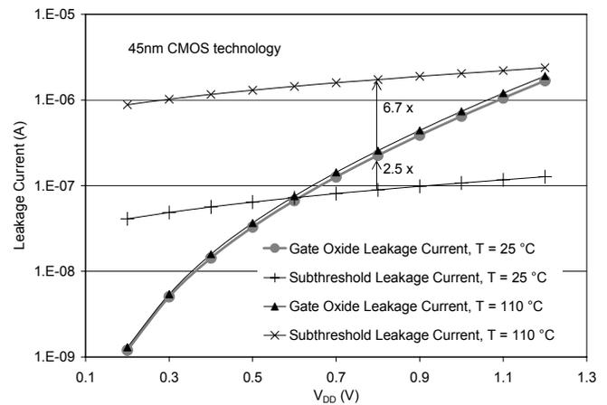
Fig. 1. Comparison of subthreshold and gate oxide leakage currents produced by an NMOS transistor for various supply voltages at two different die temperatures.  $I_{subthreshold}$ :  $V_{GS} = 0$  and  $V_{DS} = V_{DD}$ .  $I_{gate}$ :  $V_{GS} = V_{GD} = V_{GB} = V_{DD}$ .
