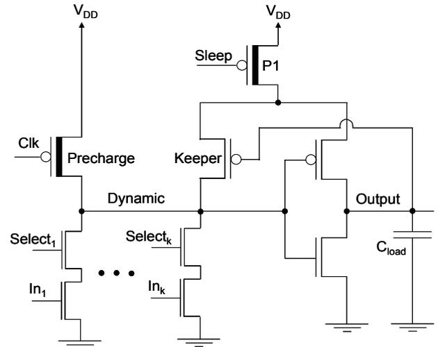
**Fig. 5. A k-bit current starved dual- $V_t$  domino multiplexer with a high- $V_t$  PMOS sleep transistor (P1). High- $V_t$  transistors are represented by a thick line in the channel region.**
