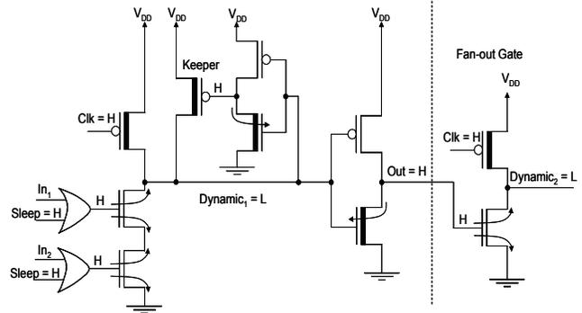
**Fig. 3. A two-input dual- $V_t$  domino AND gate with inputs gated high in sleep mode. The most significant components of gate oxide leakage current in the sleep mode are illustrated with arrows. H: high. L: low. High- $V_t$  transistors are represented by a thick line in the channel region.**
