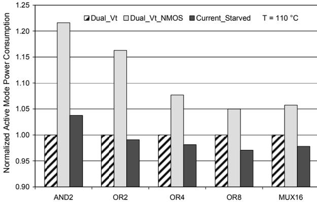
**Fig. 6. Comparison of active mode power consumption with the three domino circuit techniques. For each circuit, power consumption is normalized to the power consumed by standard dual- $V_t$  technique.**
