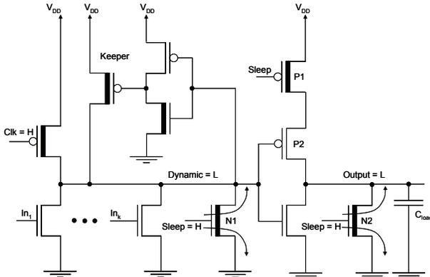
**Fig. 4. A k-input NMOS sleep switch dual- $V_t$  domino OR gate in sleep mode. Gate oxide leakage currents produced by the sleep transistors are illustrated with arrows. H: high. L: low. High- $V_t$  transistors are represented by a thick line in the channel region.**
