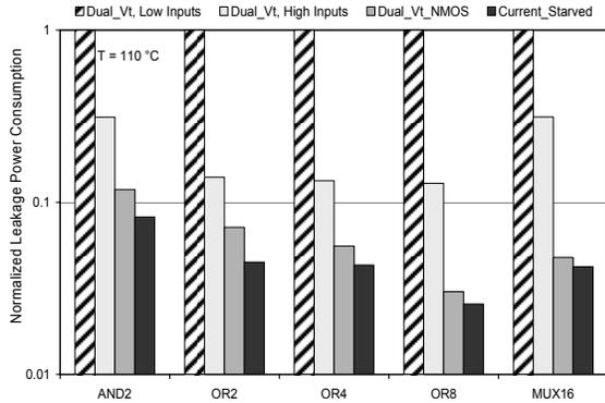
**Fig. 7. Comparison of total leakage power consumed by domino circuits with the three circuit techniques at 110 °C. For each circuit, leakage power is normalized to the leakage power of standard dual- $V_t$  technique with low inputs.**
