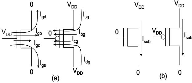
**Fig. 2. Maximum gate oxide and subthreshold leakage current states in NMOS and PMOS transistors. (a) Maximum gate oxide leakage current state. (b) Maximum subthreshold leakage current state.**
