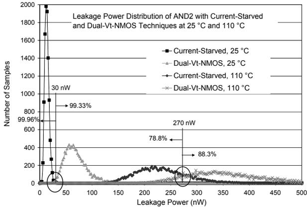
**Fig. 9. Comparison of the leakage power distributions of 2-input dual- $V_t$  domino AND gates due to process parameter variations at 110 °C and 25 °C.**
